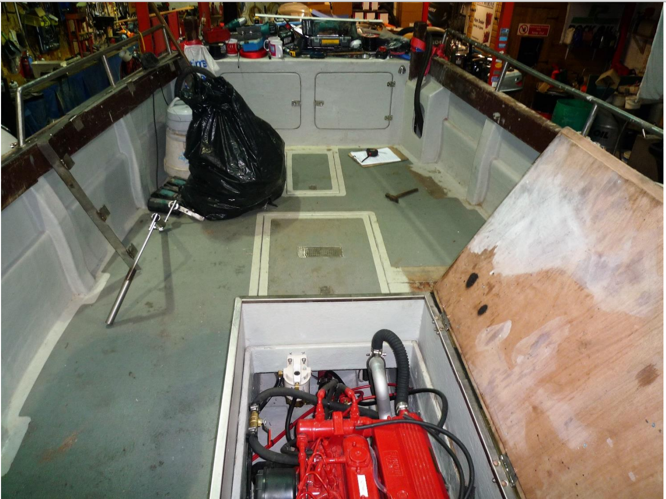
Deck layout. The batteries are stored in the locker that can be seen at the transom. The two hatches on the deck are not fitted with any retaining lanyards
