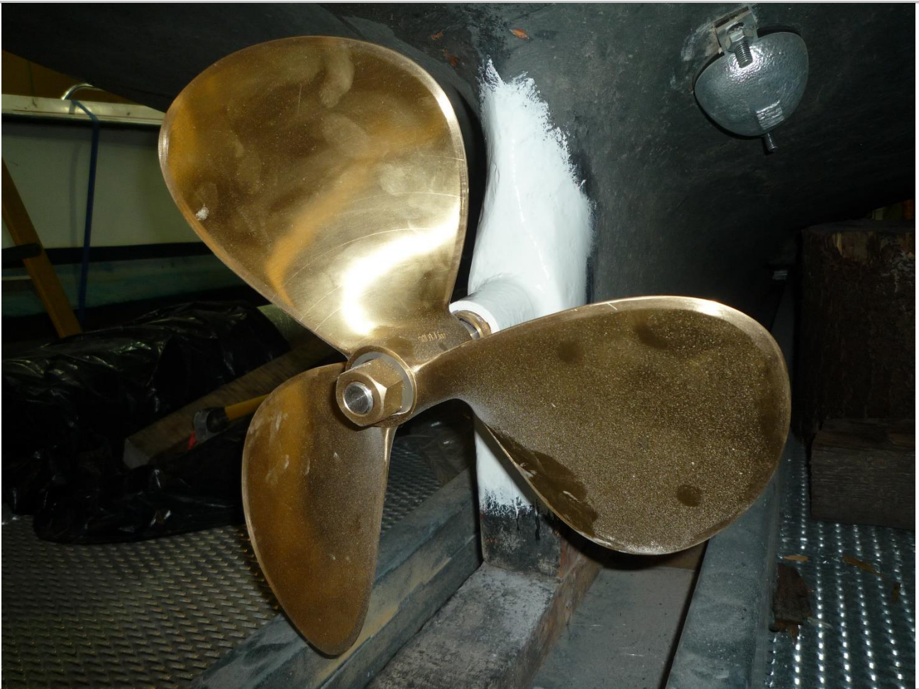
New bronze propeller and new anode can just be seen top right hand. The propeller nut is locked.
