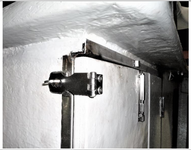
The latch on the wheelhouse door that can automatically secure the door closed if personnel are within the wheelhouse if the door is closed abruptly. It then cannot be opened from the inside.
