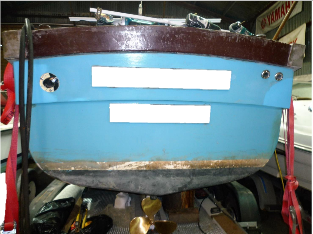
Transom showing exhaust outlet port top and bilge pump outlet starboard top.
