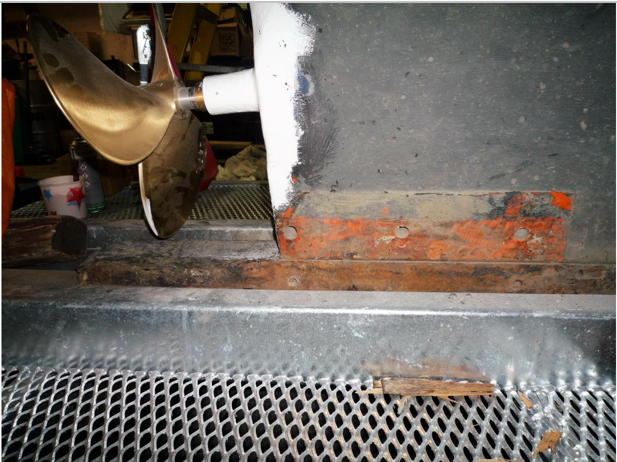
The keel extension supporting the bottom end of the rudder was not available for inspection and has not been fitted yet
